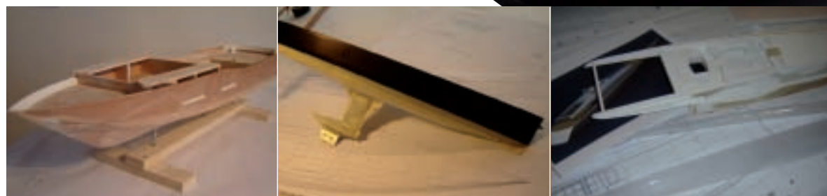
Left to right: wooden hull set in epoxy of a Peri Yacht 33; a 62cm caferacer; the synthetic superstructure for a 1:60 model of Vitruvius 200;
