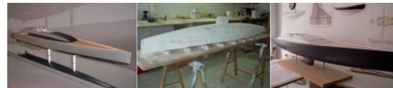
the finished model on a mirror base; a 1:33 ketch created using strip planking and cloth set in epoxy; the same model finished shows off the yacht's lines
